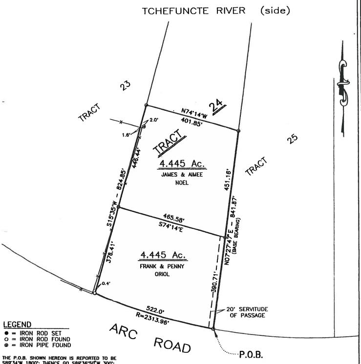
THE P.O.B. SHOWN HEREON IS REPORTED TO BE S89'34'W 1800'; THENCE GO S89'36'50'W 300'; THENCE GO ALONG A CURVE TO THE RIGHT WITH A RADIUS OF 2313.96' AND AN ARC LENGTH OF 352.9' FROM THE SECTION CORNER COMMON TO SECTIONS 38, 16 & 15, T-6-S, R-10-E, ST. TAMMANY PARISH, LOUISIANA
