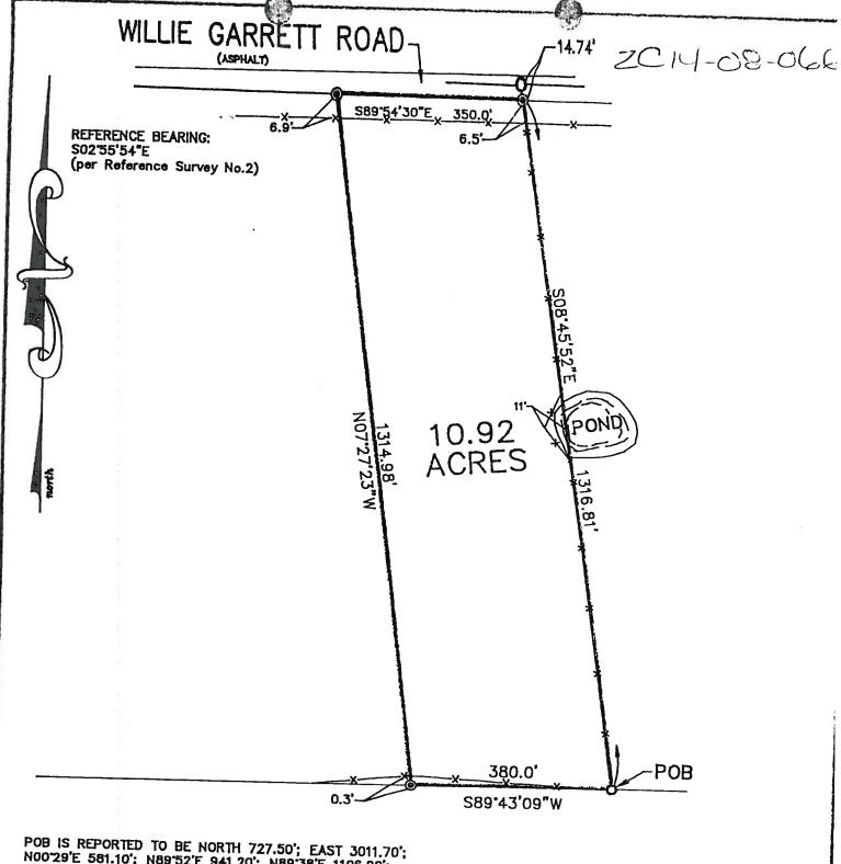
POB IS REPORTED TO BE NORTH 727.50'; EAST 3011.70'; N00'29'E 581.10'; N89'52'E 941.20'; N89'38'E 1106.90'; FROM THE SECTION CORNER COMMON TO SECTIONS 29, 30, 31, & 32, T4S, R10E.
